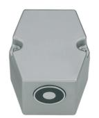
The LCN SEM7800 Series are heavy duty, electrically controlled door holding magnets. Magnets are fail safe and hold until the current is interrupted. A manual door closer is used to control and close the door. A choice of floor, recessed wall, or surface mounted wall magnets are available.
