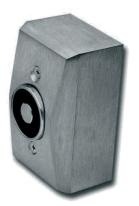
The LCN SEM7800 Series are heavy duty, electrically controlled door holding magnets. Magnets are fail safe and hold until the current is interrupted. A manual door closer is used to control and close the door. A choice of floor, recessed wall, or surface mounted wall magnets are available.
