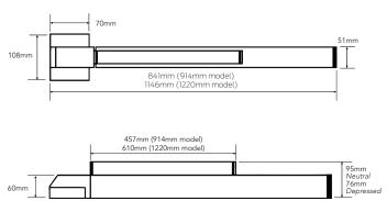
Device centre line from finished floor: 1011mm
