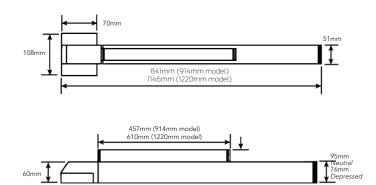
Device centre line from finished floor: 1011mm
