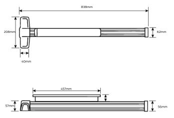
Device centre line to finished floor: 1011mm
