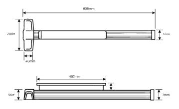
Device centre line to finished floor: 1011mm
