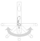
Handing of the lever is a simple operation: rotate the lever to the desired handing and then guide the spring mechanism into the channel.
