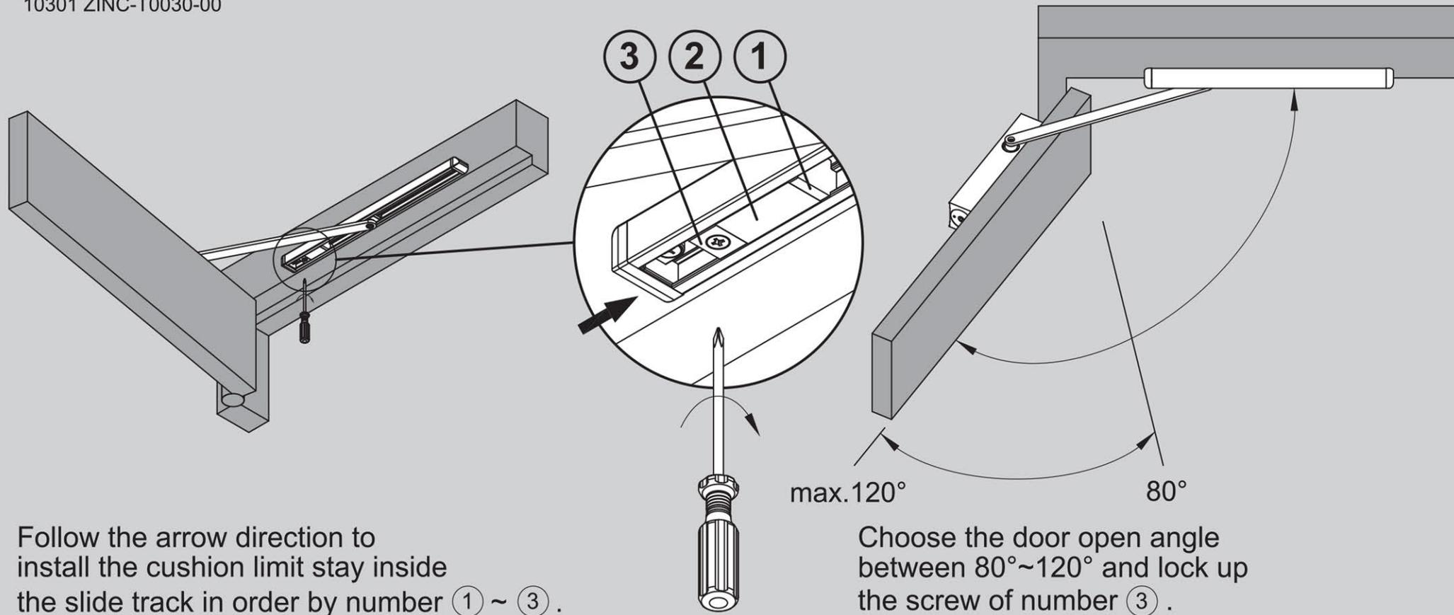
Follow the arrow direction to install the cushion limit stay inside the slide track in order by number ① ~ ③ .
