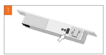
Remove the rubber cap to expose the capstan changeover wheel.
