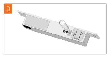
Insert a small screwdriver through the window.
