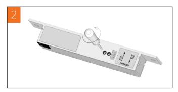
Fully loosen both the capstan release screws (screws are captured by the plastic gommet).
