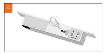
Tighten the two capstan releasing screws. Replace the rubber cap to the close window.
