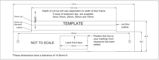
If frame is not prefabricated, use the enclosed stick-on template to prepare strike cut-out in frame. Install strike as described in diagram.
