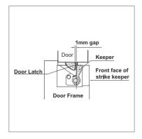
As drawn in the diagrams, there should be a 1mm gap between the door latch and the front face of the strike keeper, preventing the door from creating back pressure on the strike keeper when the door is closed.
