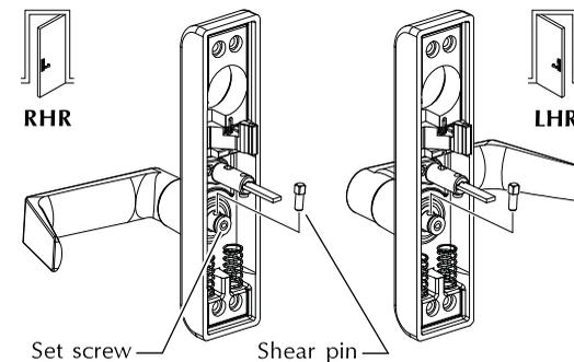
3. Install cam with "R" facing out for RHR or "L" facing out for LHR.
